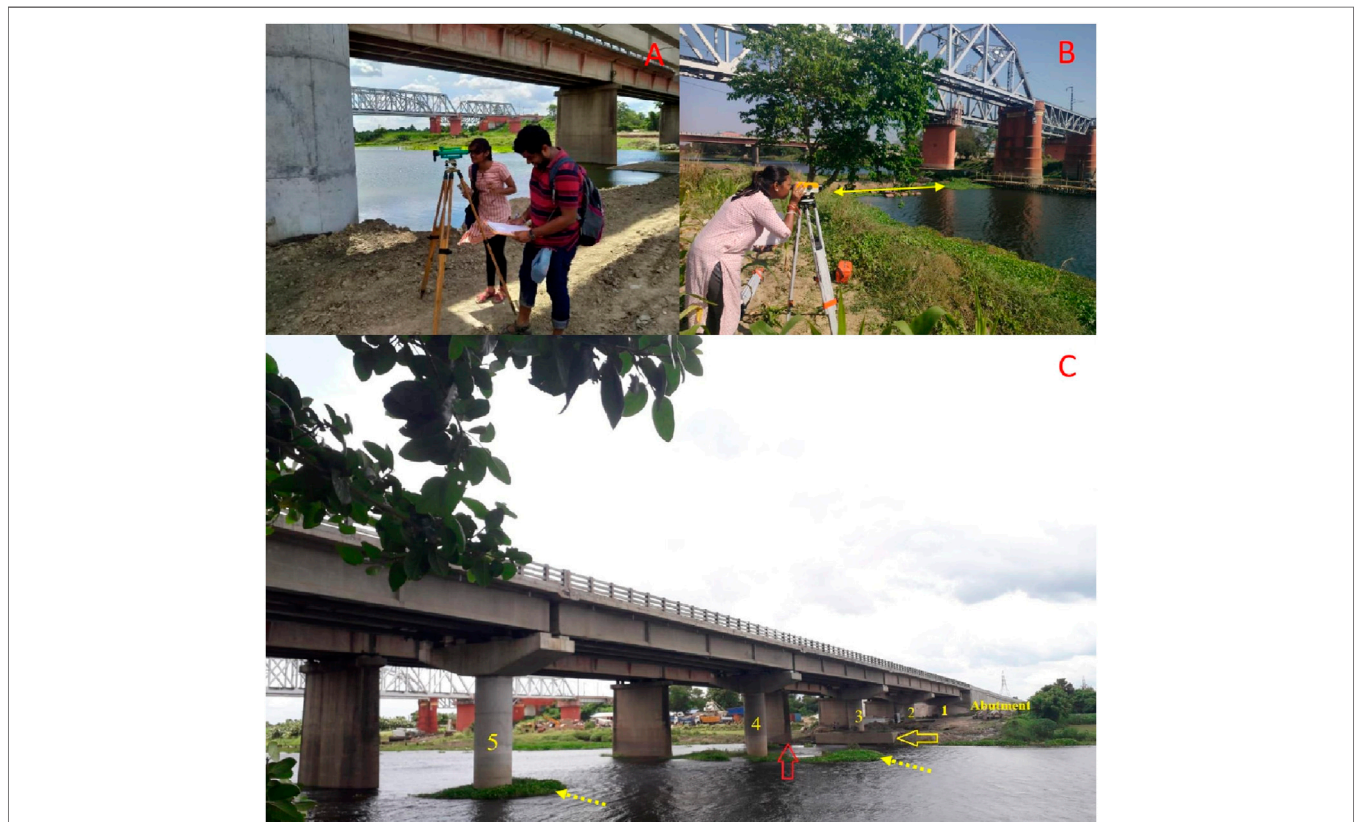
FIGURE 3 | (A) The volume of soil fill for facilitating construction processes is being estimated by Shrabani Das (co-author) and her classmate. (B) The cross-sectional morphology of the channel downstream of the 3rd railway bridge is being measured. (C) A wide yellow arrow points towards the right bank, showing a dike well above the water level of the channel as of 20.07.2024. Notably, the earth-filling from the bank to the dike has partially closed the channel. The red wide arrow points to the pier without a dike of the old bridge and the flow surrounding the pier. Dotted yellow arrows indicate the hyacinths stuck to the dikes at the base of the piers of the new bridge.
