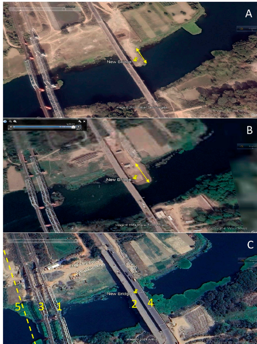
FIGURE 2 | Google Earth Pro images showing different phases of bridge constructions and interference with the channel morphology. (A) Image of December 2015 showing soil filling within the channel from the right bank. (B) Image of March 2022 showing soil filling within the channel from the right bank and diases at the base of the pier are constructed. (C) Image of April 2023 completion of the bridge. Numbers from 1 to 5 written in yellow represents the sequences of bridges on the river (2 and 4 are highway bridges and 1, 3 and 5 are railway bridges).
